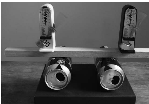
A demonstration of Huygens' clocks. The metronomes started out of phase, but became in phase after about one minute.
